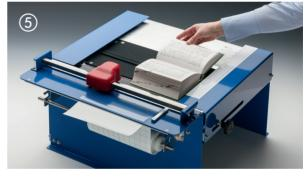
Please ensure that there is an overlap here, too, of 2 cm for the book cover. The distance between the edge and the head of the cutter should be about 2 cm. Open the book roughly at the middle and check the printed scale to see how much of the filmolux film you will need to pull off the roll.
