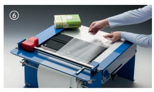
Pull the film off the roll to the measured coloured spot.
