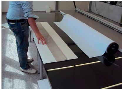
**Step 3:** Peel off the SAV so that the backing paper still lies flat on the table and the adhesive side of the SAV is facing up.
