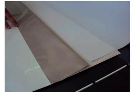
**Step 4:** Place the varitex on the backing paper close to the edge of the SAV.
