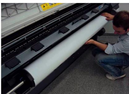
**Step 8:** Use the SAV to feed the material into the printer as usual.
