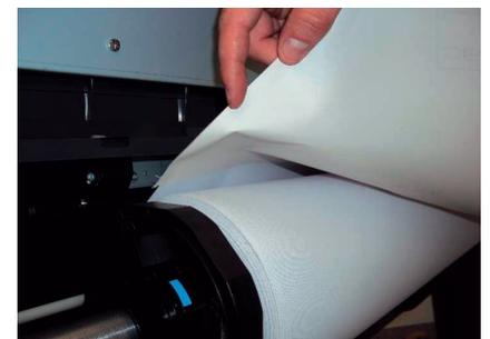
**Step 7:** Put the roll into the printer. Note: the varitex needs to be in between the SAV and the backing paper.
