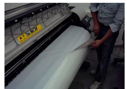
**Step 10:** Remove the SAV. fold back onto the backing paper and store for later use.
